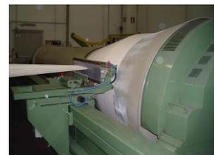
Once the beam is full, it is taken to one of Parà's ultra-modern "airjet" looms where a weft (horizontal yarn) is woven across it. This critical process makes a cloth that needs to be strong and slightly elastic. Only the highest quality yarns ensure this. The "loomstate" fabric is then washed to remove any lubricants and impurities, and is then ready for further processes, depending on requirements.
