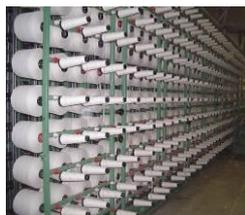
The first stage of any weaving production is "beaming" where the warp (vertical yarn set) is wound onto a giant spool. This is done by placing thousands of cones of yarn on a rack called a "creel" and placing each yarn carefully so that it is in exactly the right location on the beam. This is how a perfectly regular stripe effect is made. Parà has 7 beaming machines for great capacity and flexibility.
